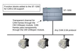
Slave devices connected via a CAN 2.0A based protocol
