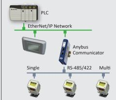
The Communicator works as a serial Modbus RTU master to the connected slave devices, and as a slave towards the PLC
