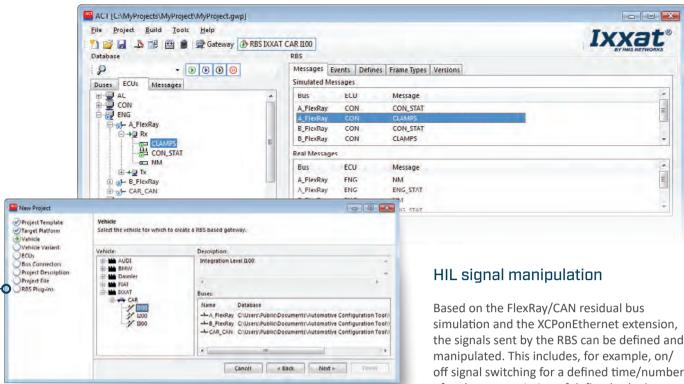
Based on the FlexRay/CAN residual bus simulation and the XCPonEthernet extension, the signals sent by the RBS can be defined and manipulated. This includes, for example, on/ off signal switching for a defined time/number of cycles, transmission of defined substitute values with switched-off signals and defined corrupting of CRCs and alive counters for all signals sent by the RBS. Signal manipulation control can be done via user code, the gateway or XCPonEthernet.
