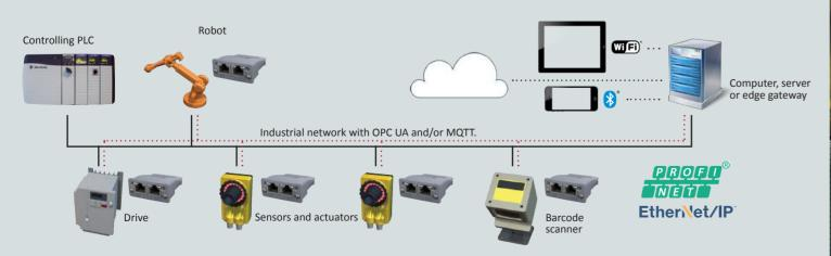
With OPC UA or MQTT communication on the factory floor, it is possible to use a computer, server or edge gateway to relay information to IT systems and clouds. Anybus CompactCom enables devices and machines on the factory floor to communicate with any industrial network using OPC UA or MQTT.
