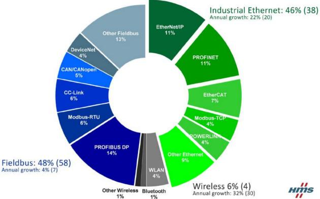
We see that industrial Ethernet and Wireless technology growth is accelerated by the increasing need for industrial devices to get connected and the Industrial Internet of Things. Industrial Ethernet now accounts for 46% of the market (38% last year). Wireless technologies are also coming on strong, now at 6% (4) market share. Combined, industrial Ethernet and Wireless now account for 52% of the market, while traditional fieldbuses are at 48%.
