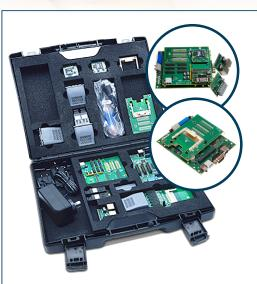
The HMS Starterkit case includes all the additional boards, adapters and cables needed to try and evaluate Anybus CompactCom. The actual CompactCom modules and bricks are ordered separately.
